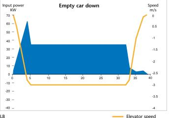
Car size: 1600 kg | Speed: 3m/s, 0.8m/s | Travel: 100 m | Machinery: MX18 + MLB
